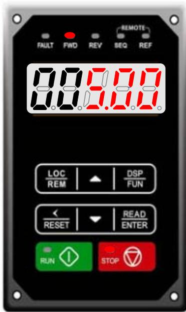
Fig 5.1: LED Keypad (Stopped)
